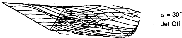
Fig. 4 Vortex model of the leading- and trailing-edge wakes after 15 steps (only longitudinal segments are shown since in this case of steady-state flow, the strength of the spanwise elements is zero).
